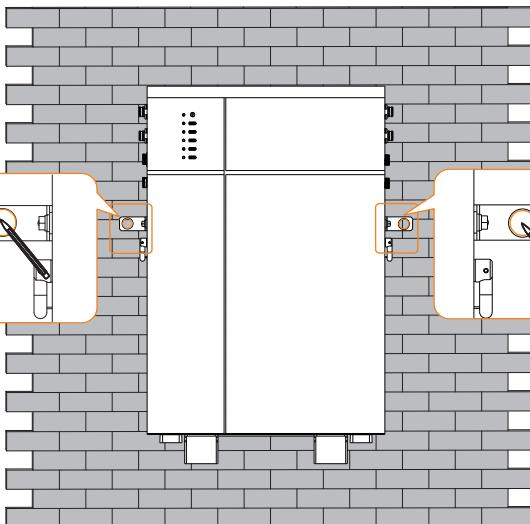
Draw two circles, with one on each side. Gently carry the battery module down to the ground.
