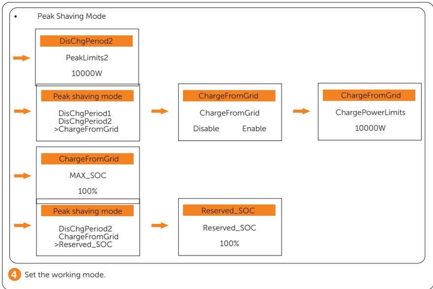
\* In the TOU mode, different working modes, i.e Self-use, Charging, Discharging, Peaking shaving and Battery off can be set for different time periods in accordance with actual needs and environment conditions through SolaX Cloud App or Web. Please refer to Web Guide or App Guide for details about how to set the TOU mode.
