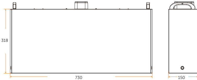
Figure 2-8 Dimension: Battery module (TP-HS50E)
