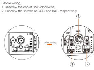
① Insert the orange power cable into the orange socket (2) Insert the black power cable into the black socket ③ Screw the communication cable into the communication socket
