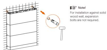
Step 7: Align the wall brackets to the wall based on the hole marks, insert two ST6\*55 self-tapping screws (TP-HS50: part B) and two washers (TP-HS50: part C) into the holes, and then use a torch wrench (extender length: at least 9.84 inch/250 mm) to secure them.
