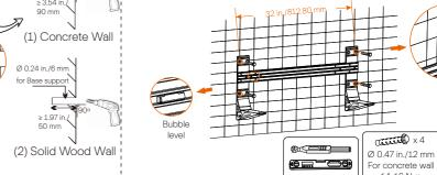
20-25 N·m 14-16 N·r Note: The bubble level on the transverse plate can be used as an auxiliary tool, additionally, please prepare a spirit level to measure whether the plate is even or not. (2) Place the Base onto the assembled base support, and then secure both sides with four
