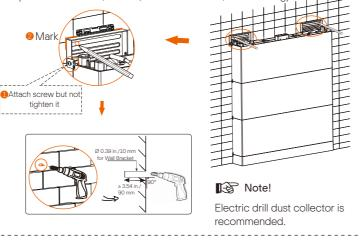
Step 6 (Optional): Hammer in the expansion bolts (TP-HS50: part D) into the holes.
