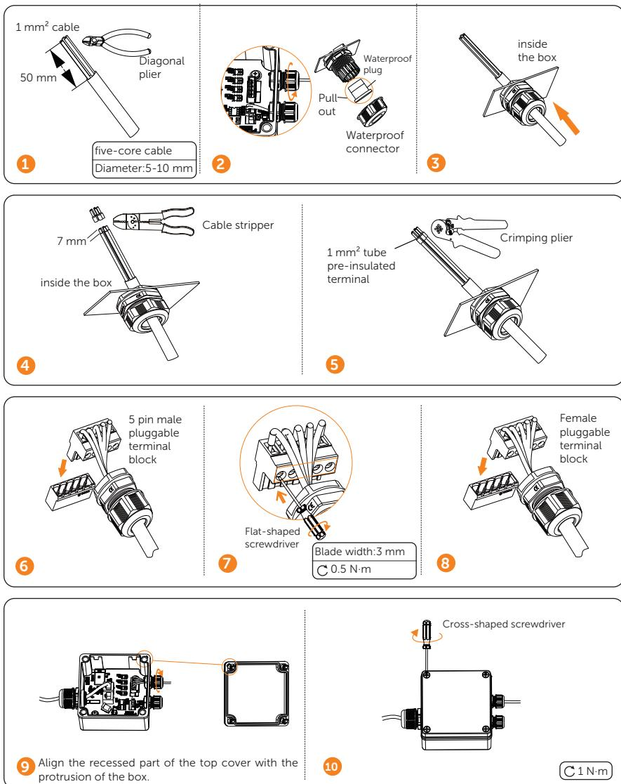
b) DO port connection under the control of SG Ready
