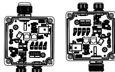
Waterproof connectors installed upwards or downwards
