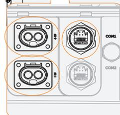
\* Regardless of how many battery modules installed, please put a waterproof cap on the communication port of the unconnected port of battery module.
