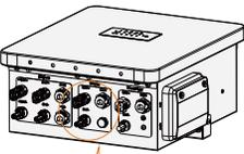
Parallel box Slave "BAT+", Slave "Heat+" to HV10230 "B+";
