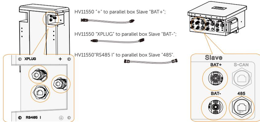
\* If there is(are) a port(s) that is(are) not wired after wiring is completed, please don't forget to put the waterproof cap(s) on the port(s).
