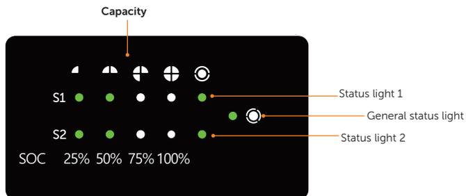
The LED indicators on the front panel of the BMS and the battery modules indicate the operating status. Description of the status indicators of BMS is shown as follows:
