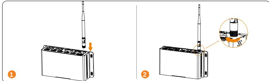
Connection through SMA-F connector (Applicable only to cabinet installation):
