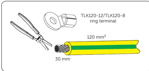
Figure 7-5 Striping cable jacket
