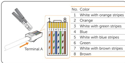
Figure 7-49 Crimping RJ45
