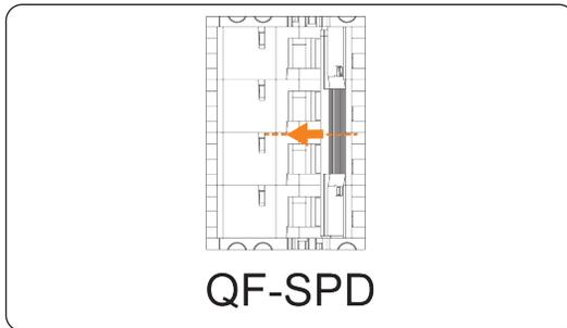
Figure 10-7 Flipping down SPD breaker
