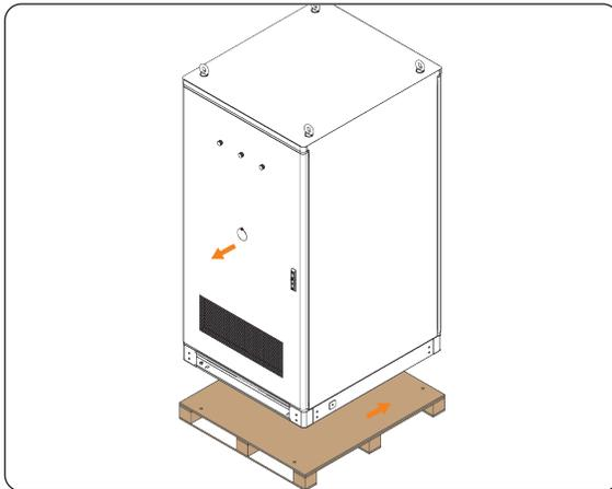
Figure 6-13 Unscrewing the screws for securing pallet
