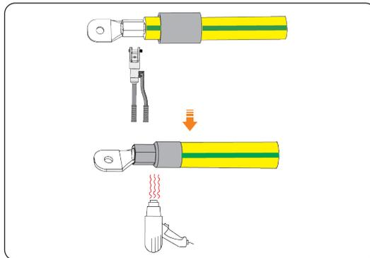
Figure 7-7 Crimping and heating
