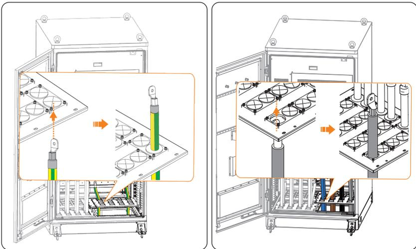
Figure 7-20 Threading through cables
