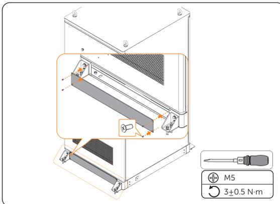
Figure 6-23 Reattaching the covers
