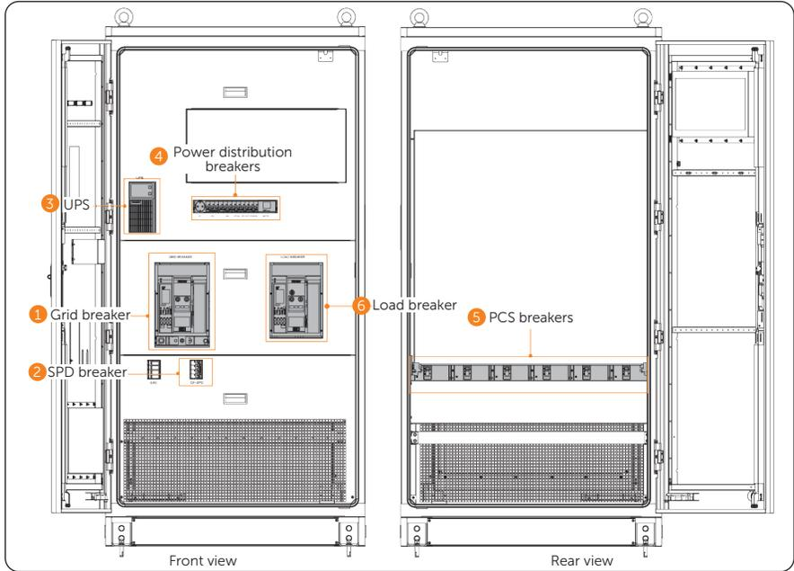
Figure 8-1 Position of modules for powering on system
