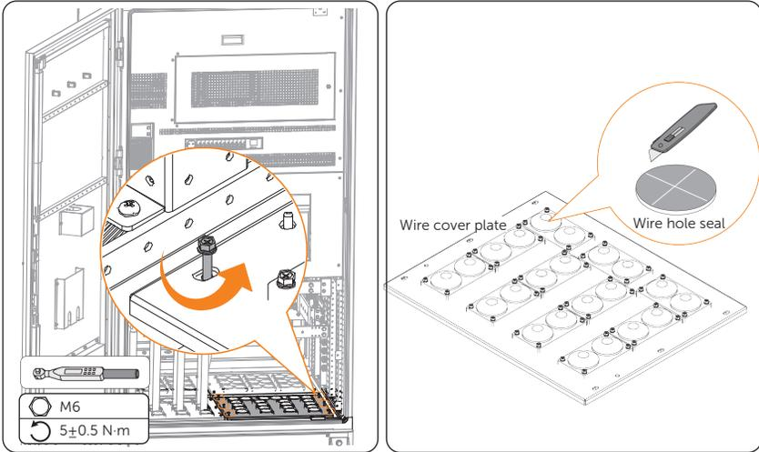
Figure 7-19 Cutting through wire hole seals
