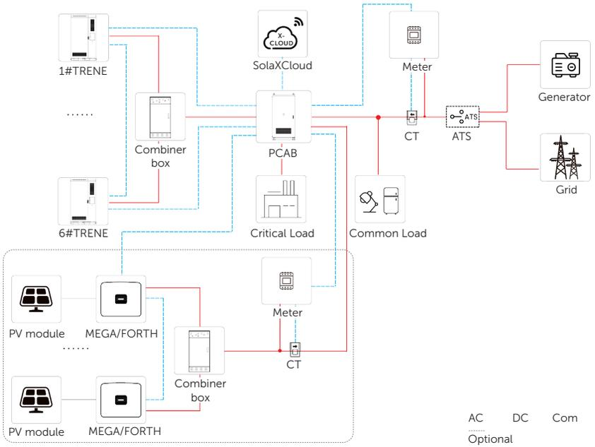
Figure 12-10 PV, DG and TRENE energy storage system overview diagram (2)
