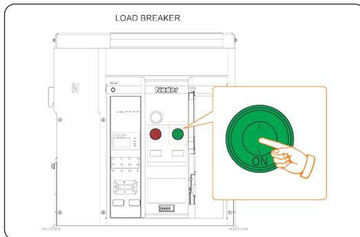
Figure 8-7 Starting the load breaker
