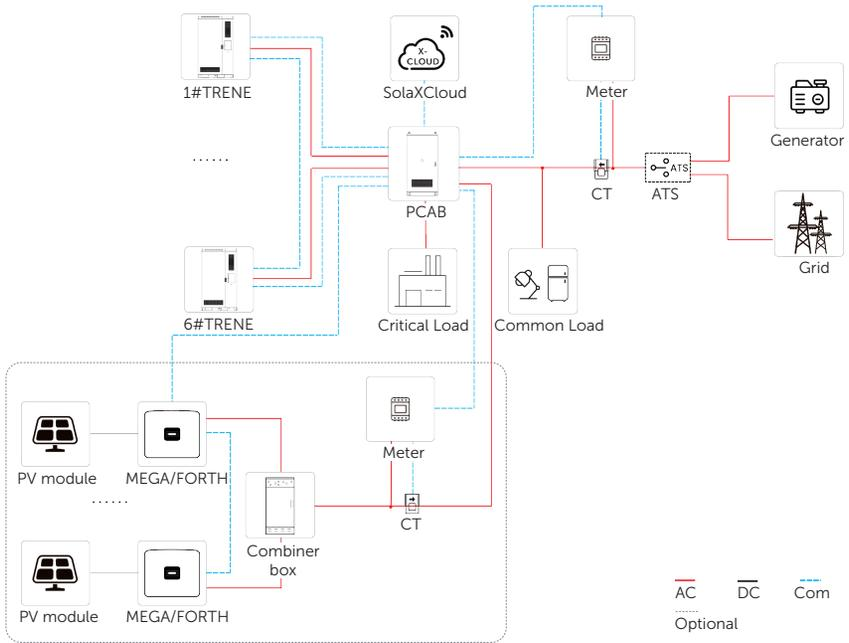
Figure 12-8 PV, DG and TRENE energy storage system overview diagram (1)
