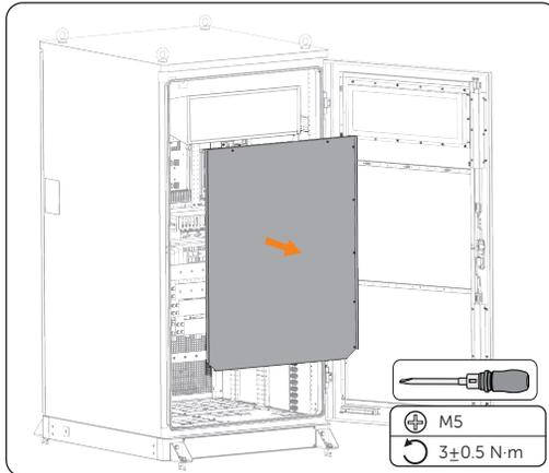
Figure 7-35 Removing the rear cover
