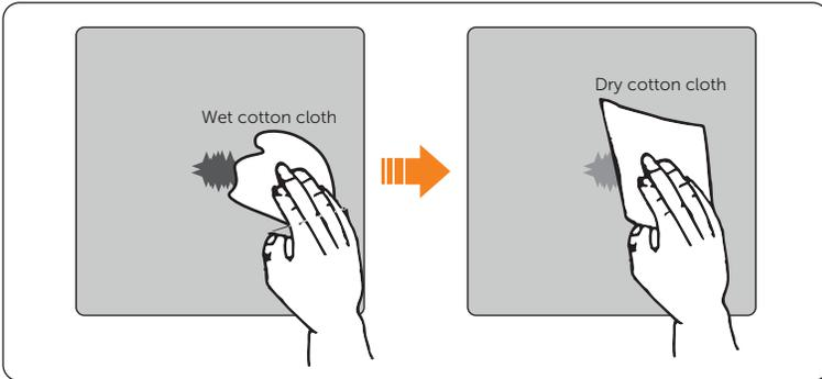
Figure 12-17 Cleaning the scratched area
