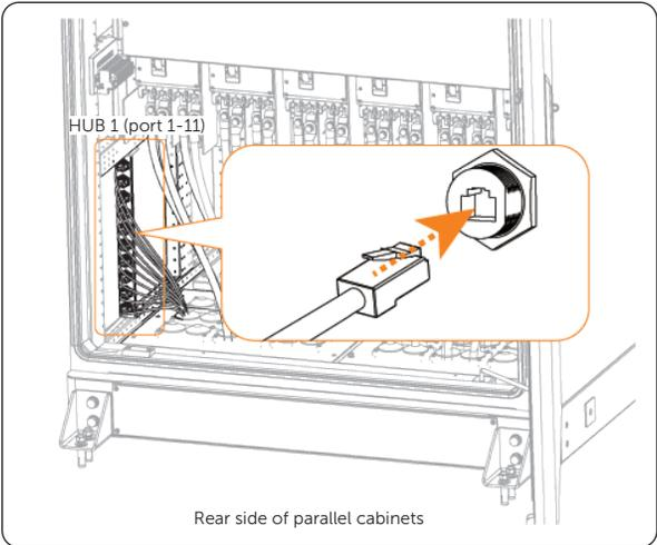
Figure 7-65 Connection to the switching cabinet
