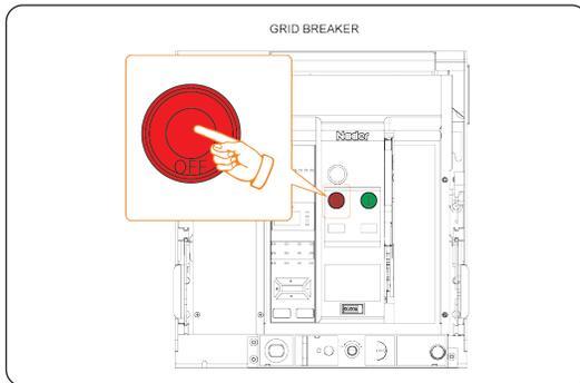
Figure 10-8 Turning off the grid breaker
