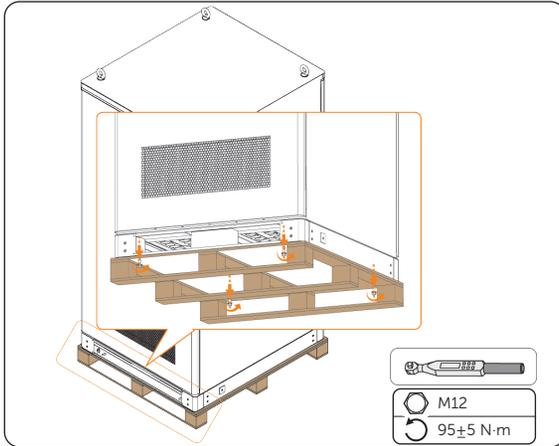
Figure 6-12 Unscrewing the screws for securing pallet
