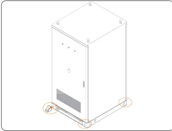
Figure 6-18 Aligning and drawing circles
