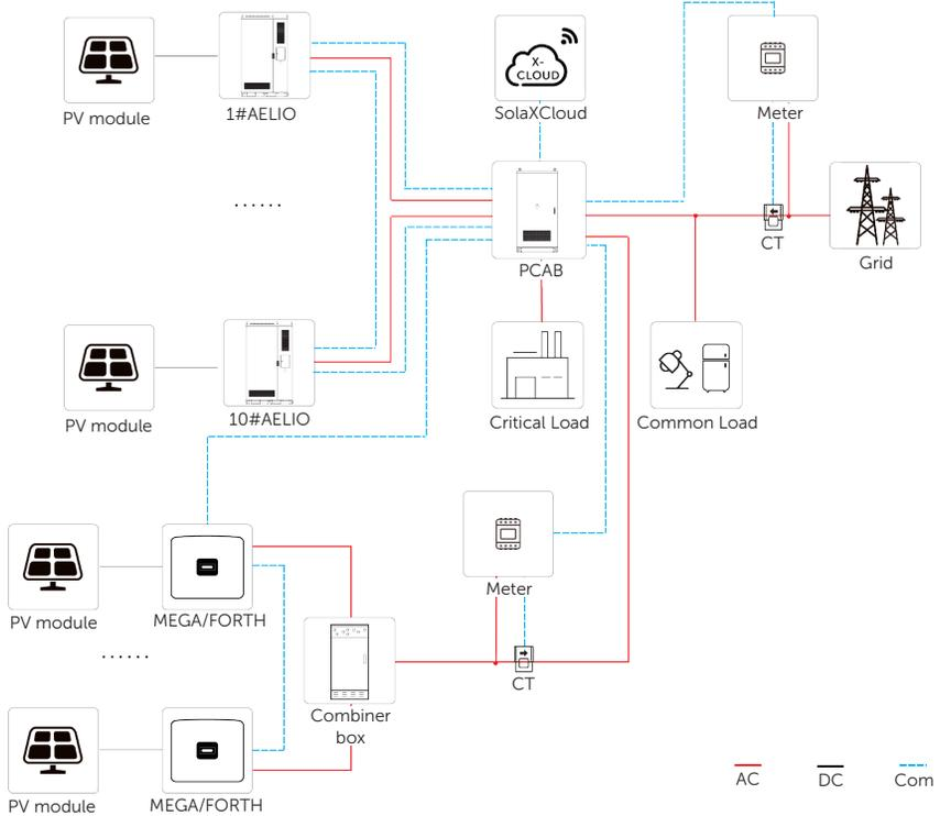
Figure 12-2 PV and AELIO energy storage system overview diagram (1)
