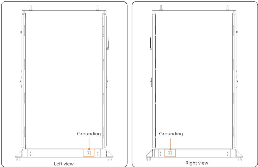
Figure 7-1 Position of the cabinet grounding terminals
