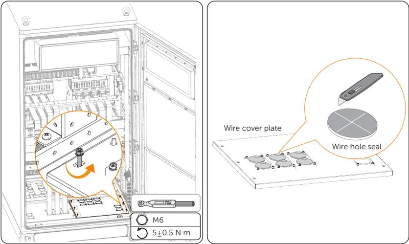
Figure 7-40 Cutting through wire hole seals
