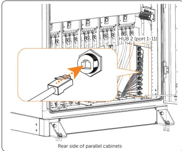
Figure 7-69 Connection to the switching cabinet
