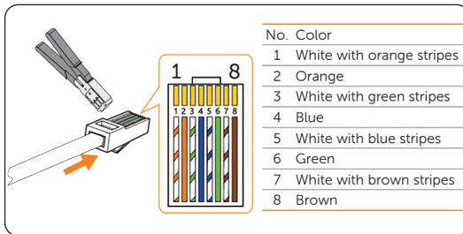
Figure 7-67 Crimping RJ45
