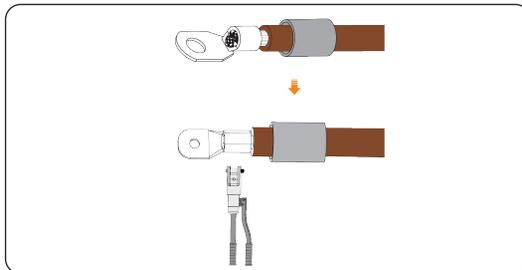
Figure 7-10 Crimping the wires and terminal
