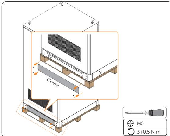
Figure 6-11 Unscrewing the screws for the cover
