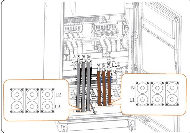
Figure 7-32 Terminal bar distribution for ESS connection
