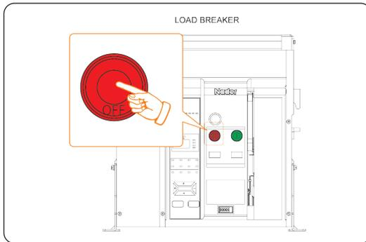
Figure 10-3 Turning off the load breaker
