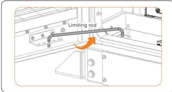
Figure 7-34 Placing the limiting rod
