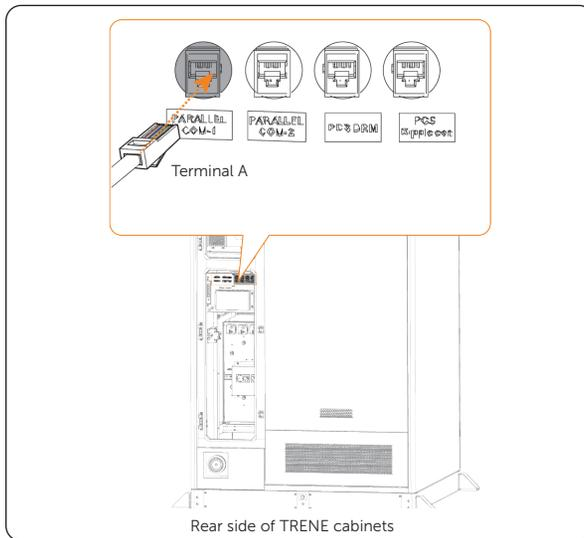
Figure 7-51 Connection to TRENE system
