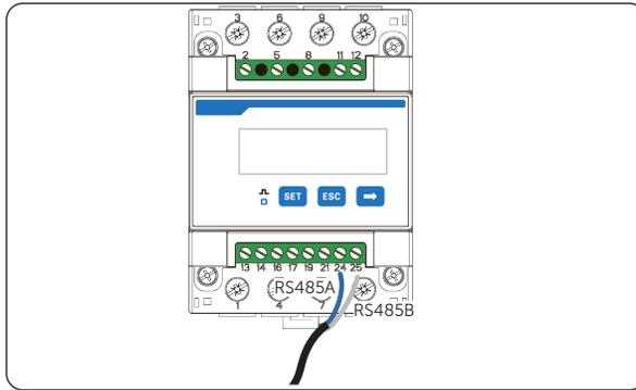
Figure 7-47 Connecting the meter
