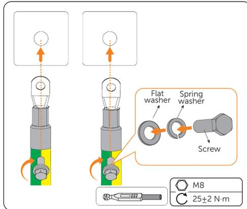
Figure 7-21 Securing the PE cable for load
