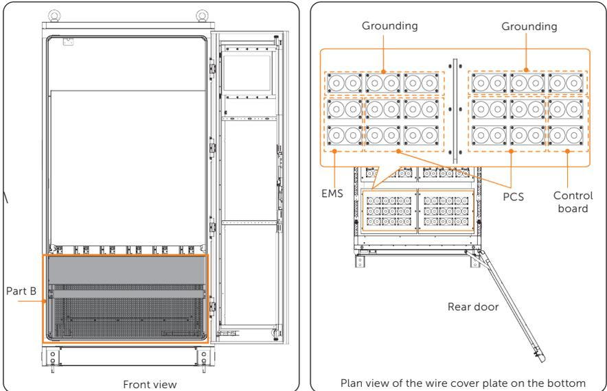
Figure 7-3 Position of PCS connection terminals
