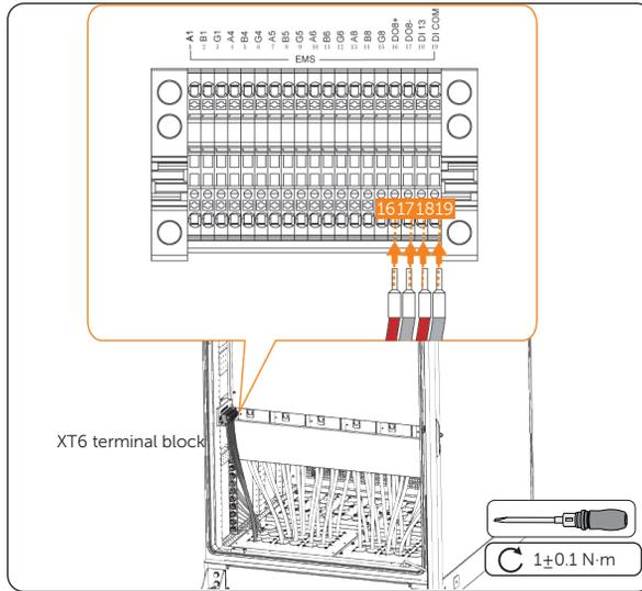
Figure 12-15 Connecting the switching cabinet
