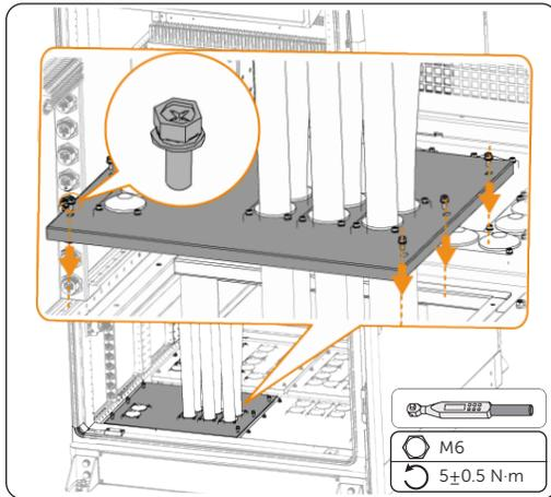
Figure 7-39 Securing plate
