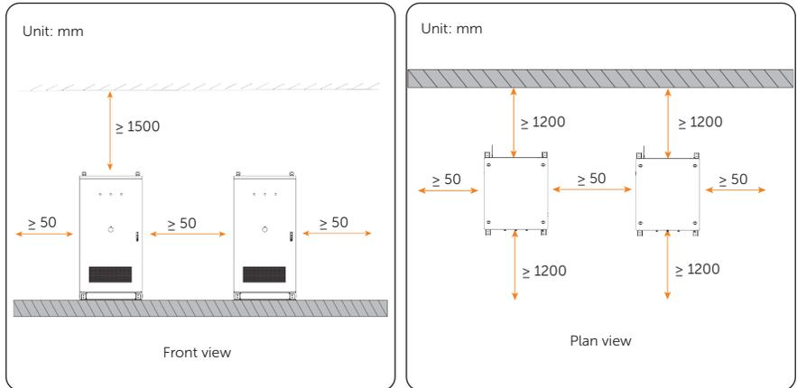
Figure 4-5 Clearance requirements for multiple cabinets
