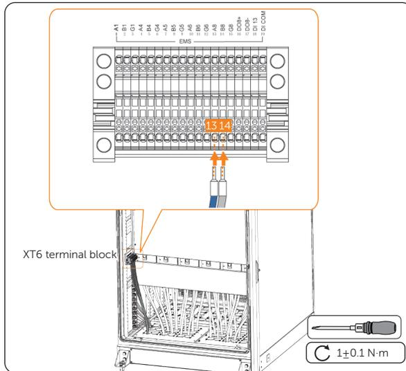
Figure 7-46 Connecting the switching cabinet
