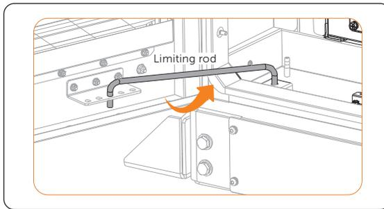
Figure 7-14 Placing the limiting rod
