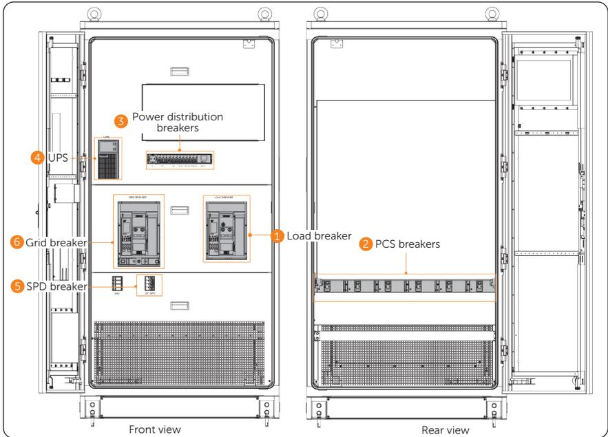
Figure 10-1 Position of modules for normally powering off the system
