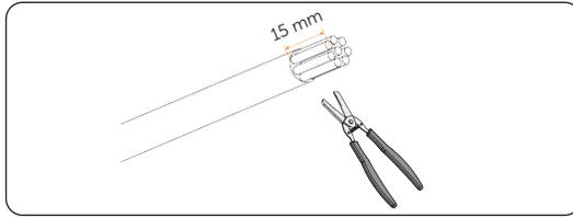
Figure 7-62 Stripping cable jacket
