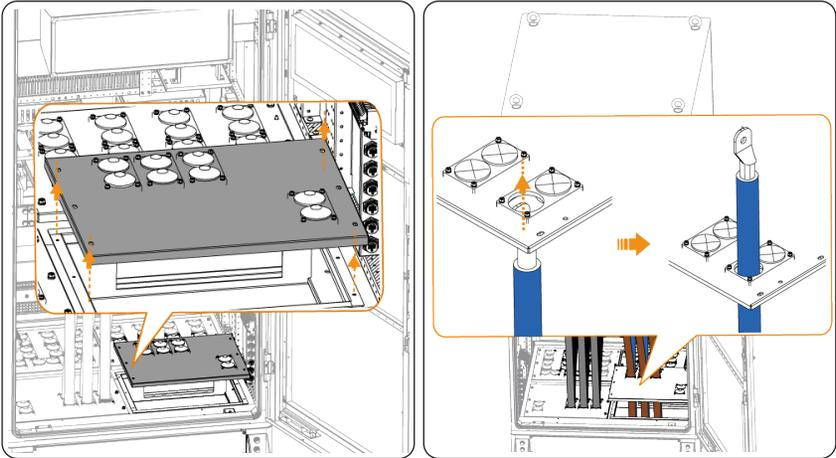
Figure 7-41 Threading cable
