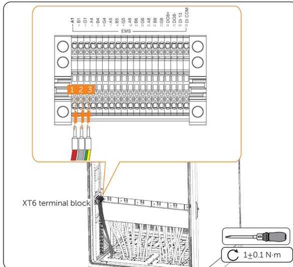
Figure 12-7 Connecting the switching cabinet
