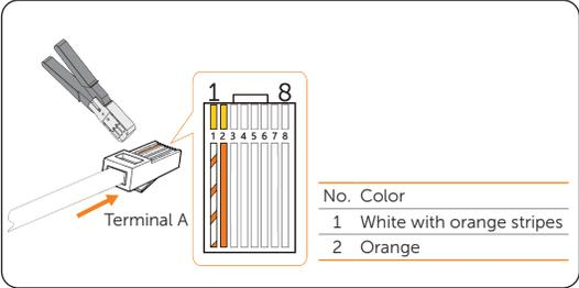
Figure 7-54 Crimping RJ45
