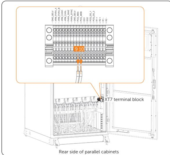
Figure 7-57 Connection to the switching cabinet
