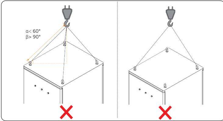
Figure 6-15 Improper way of hoisting
