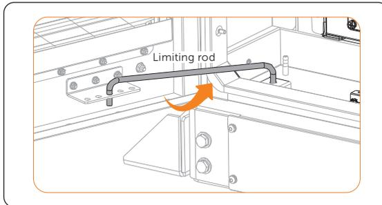
Figure 7-25 Placing the limiting rod
