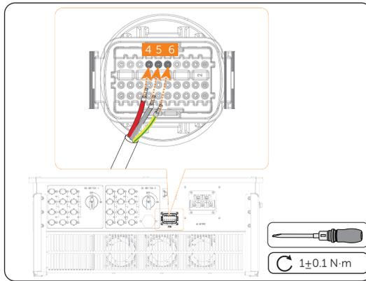
Figure 12-6 Connecting the PV inverter
