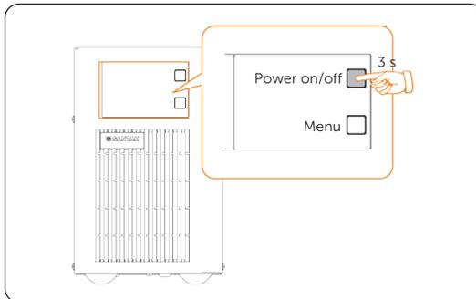
Figure 10-6 Turning off the UPS
