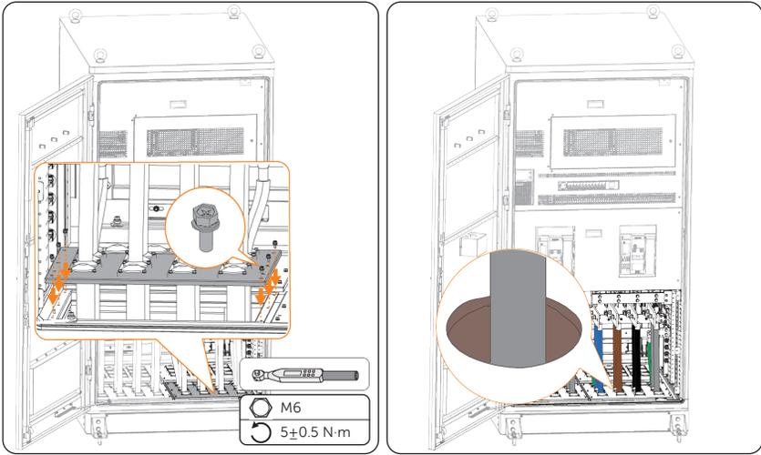
Figure 7-23 Securing plate and attaching fireproof mud
