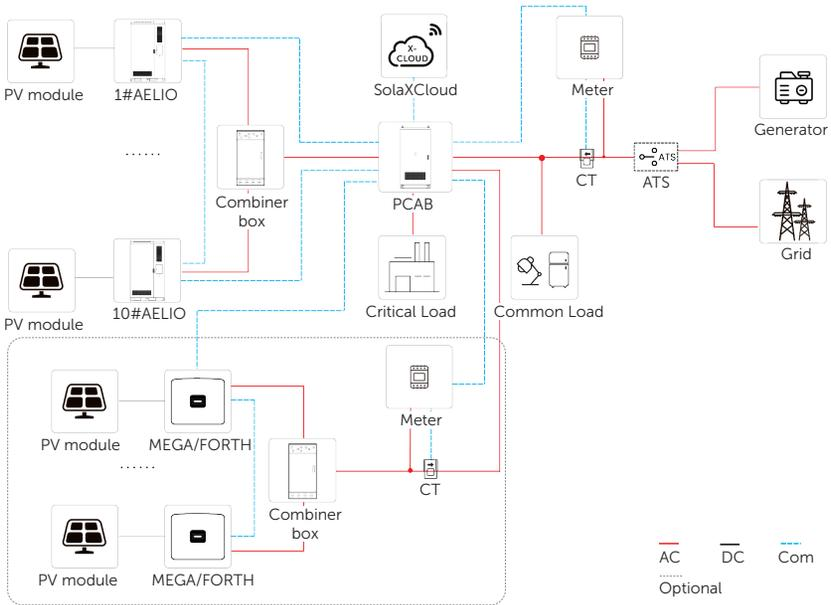
Figure 12-11 PV, DG and AELIO energy storage system overview diagram (2)
