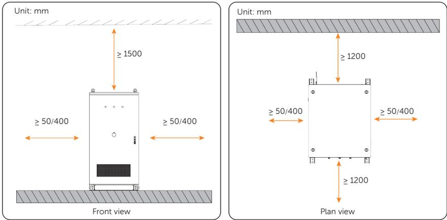
Figure 4-4 Clearance requirements for a single cabinet
