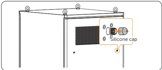
Figure 6-24 Removing silicone cap
