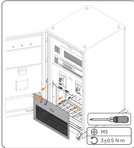
Figure 7-15 Removing the front cable cover
