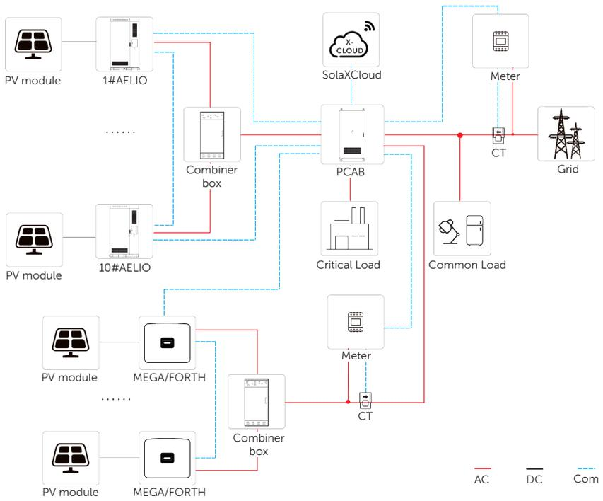
Figure 12-4 PV and AELIO energy storage system overview diagram (2)
