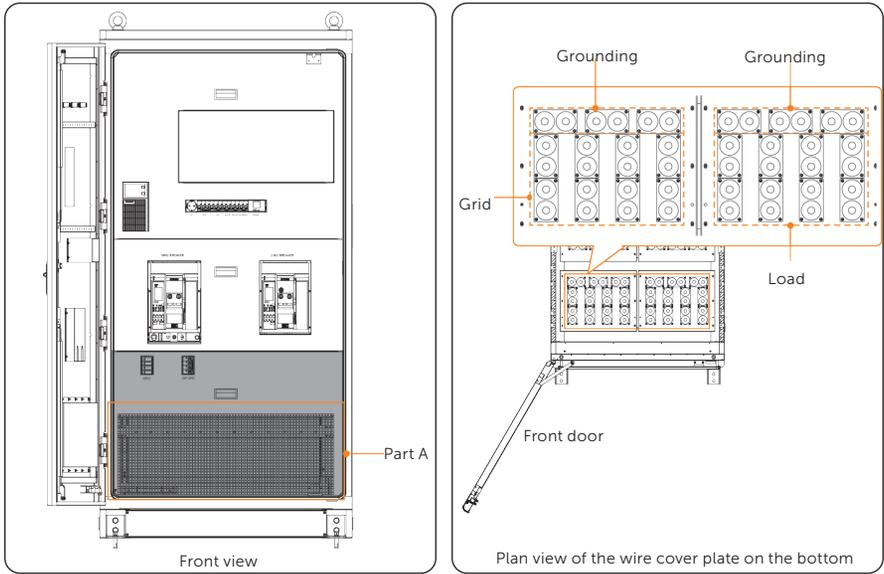
Figure 7-2 Position of grid and load connection terminals
