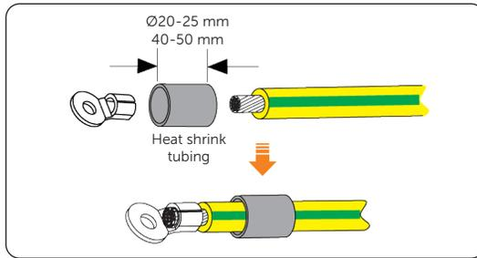
Figure 7-6 Attaching tubing and ring terminal
