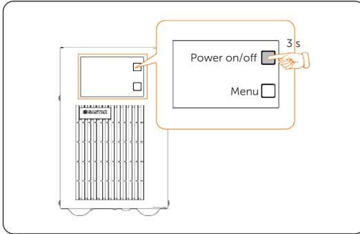
Figure 8-4 Turning on the UPS
