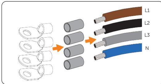
Figure 7-9 Attaching tubings and ring terminals
