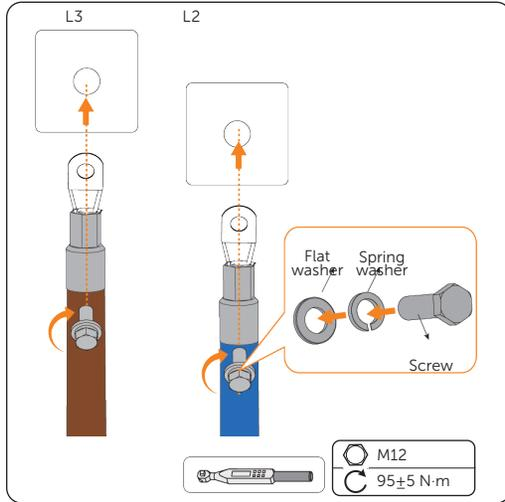
Figure 7-42 Securing L2 and L3
