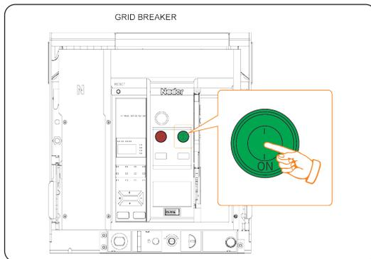
Figure 8-2 Starting the grid breaker
