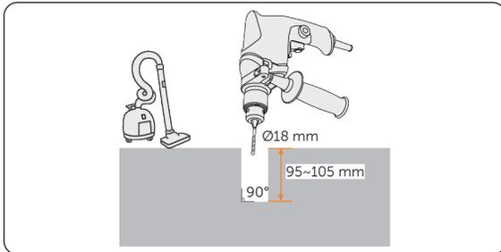
Figure 6-20 Drilling holes
