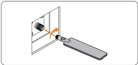
Figure 6-25 Installing antenna stick
