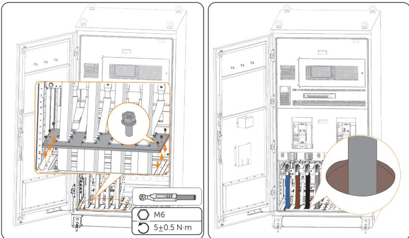
Figure 7-18 Securing plate and attaching fireproof mud
