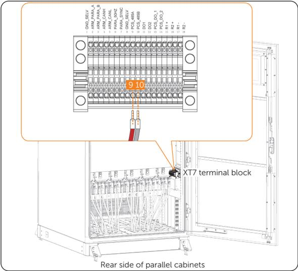
Figure 7-61 Connection to the switching cabinet
