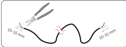
Figure 7-44 Stripping the communication cable
