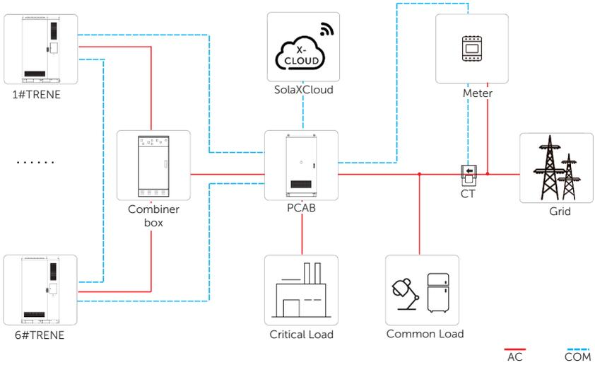
Figure 2-15 TRENE system overview diagram (2)
