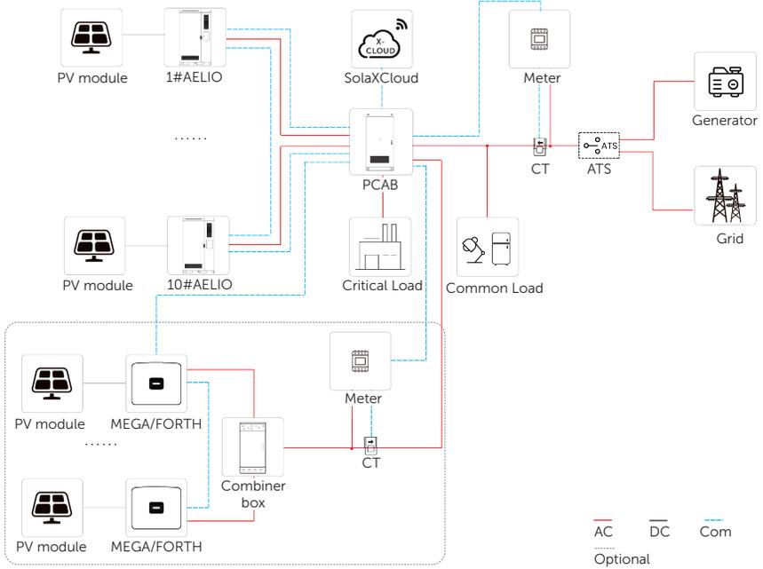
Figure 12-9 PV, DG and AELIO energy storage system overview diagram (1)
