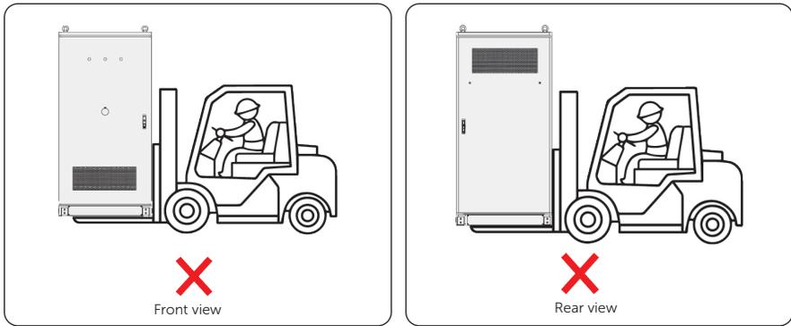
Figure 6-17 Improper way of handling
