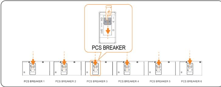
Figure 10-4 Flipping down PCS breakers
