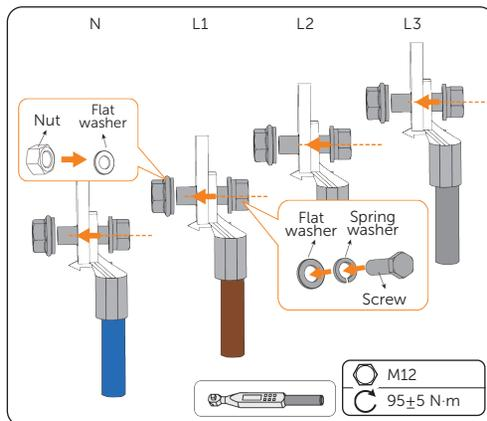
Figure 7-22 Securing the power cables for load
