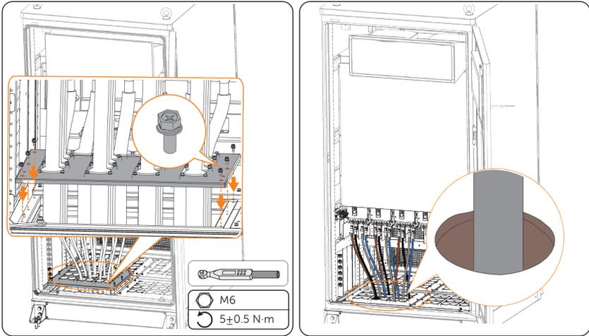
Figure 7-30 Securing plate and attaching fireproof mud
