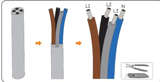
Figure 7-8 Stripping wires
