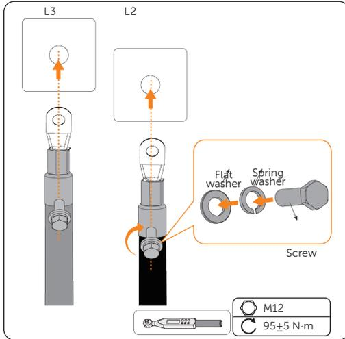
Figure 7-38 Securing L2 and L3
