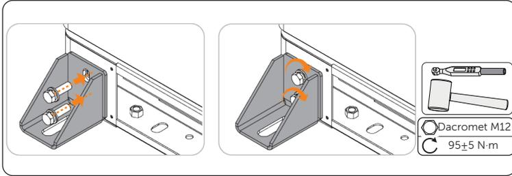
Figure 6-21 Securing the cabinet
