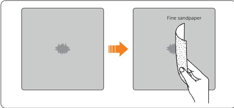
Figure 12-16 Sanding the scratched area
