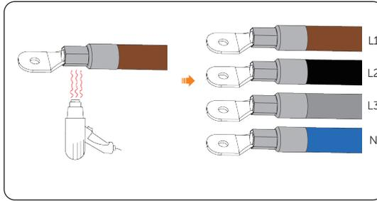
Figure 7-11 Heating the terminals
