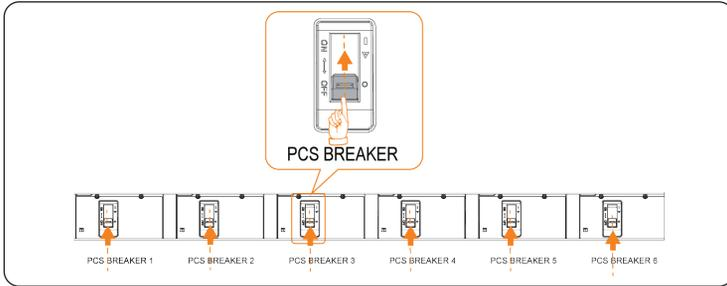
Figure 8-6 Flipping up PCS breakers
