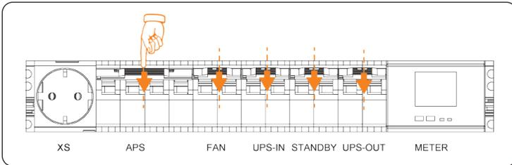
Figure 10-5 Flipping down power distribution breakers
