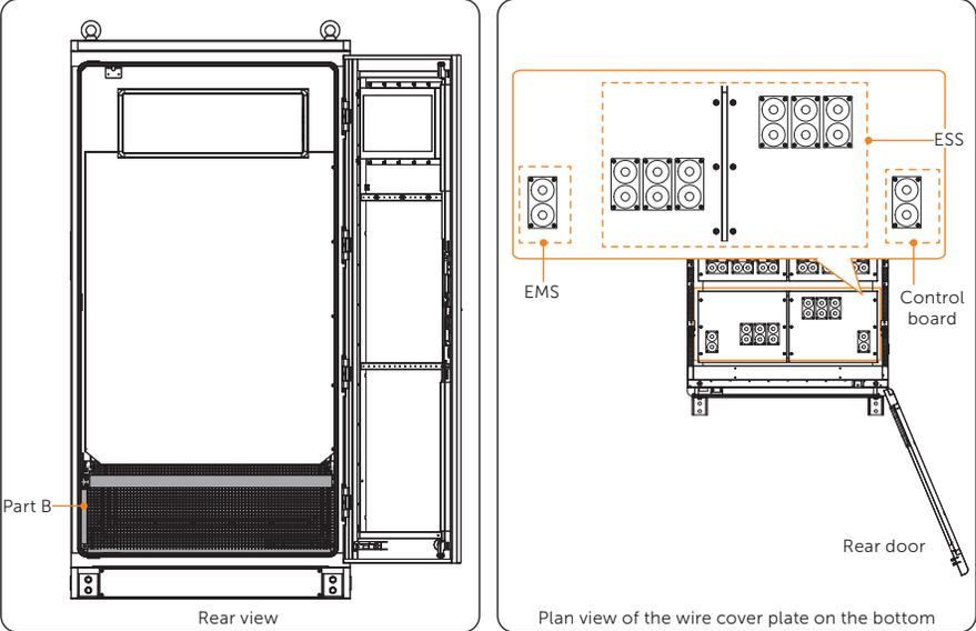
Figure 7-4 Position of ESS connection terminals
