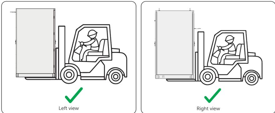
Figure 6-16 Proper way of handling
