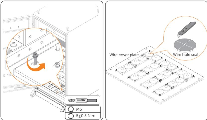
Figure 7-16 Cutting through wire hole seals
