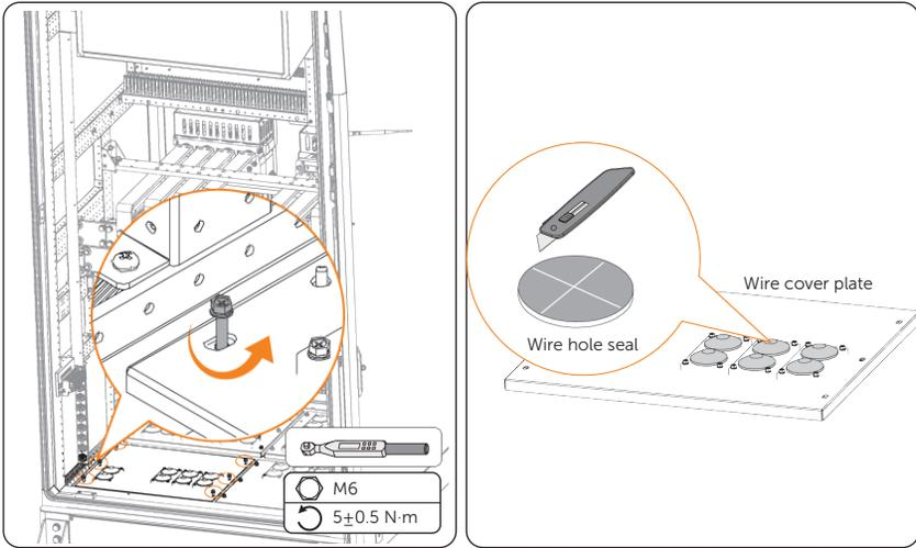
Figure 7-36 Cutting through wire hole seals
