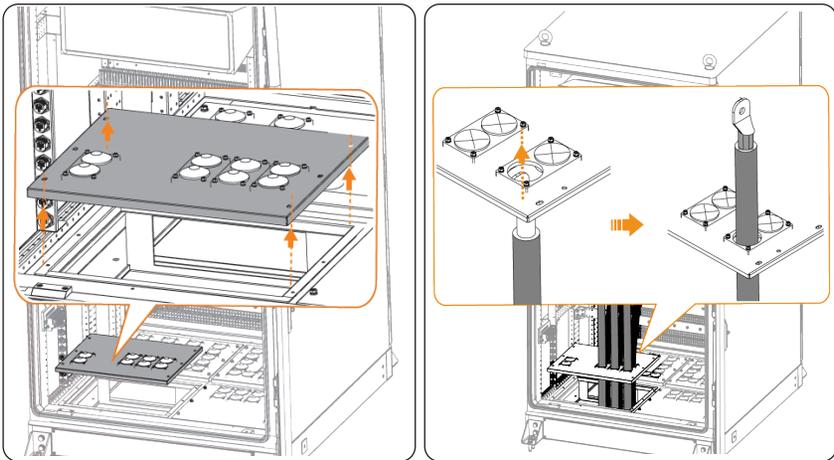
Figure 7-37 Threading through L2 and L3 cables
