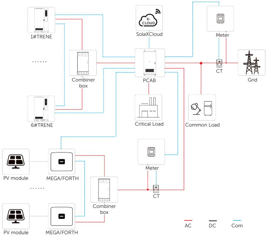
Figure 12-3 PV and TRENE energy storage system overview diagram (2)
