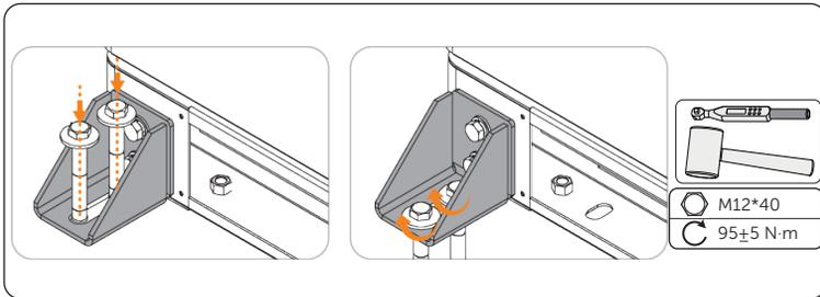
Figure 6-22 Securing the angle supports
