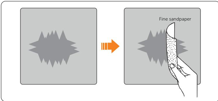
Figure 12-19 Sanding the scratched area
