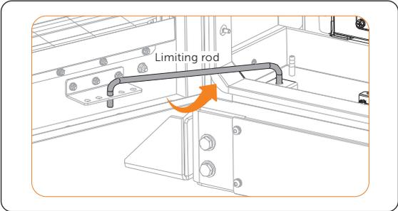
Figure 5-10 Placing the limiting rod
