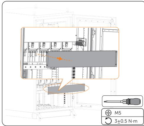
Figure 7-26 Removing the rear cover
