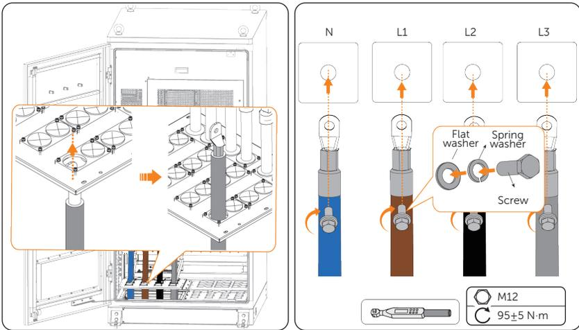
Figure 7-17 Threading and securing cables
