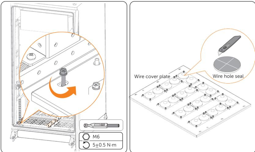
Figure 7-27 Cutting through wire hole seals
