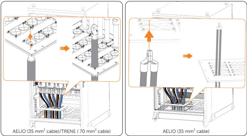
Figure 7-28 Threading through cables
