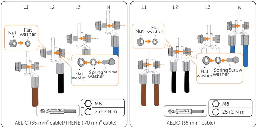
Figure 7-29 Securing cables
