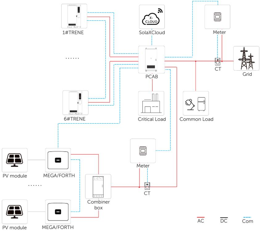
Figure 12-1 PV and TRENE energy storage system overview diagram (1)
