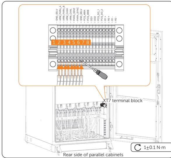
Figure 7-52 Connection to the switching cabinet
