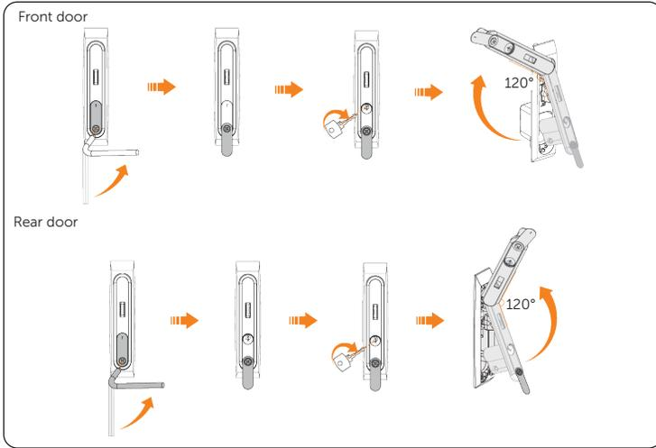
Figure 10-2 Opening the front and rear doors
