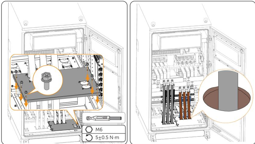
Figure 7-43 Securing plate and attaching fireproof mud
