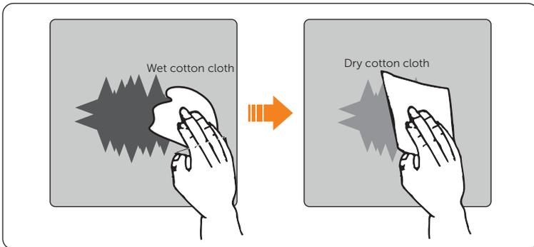
Figure 12-20 Cleaning the scratched area
