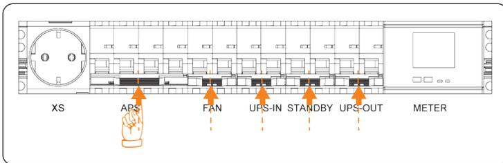
Figure 8-5 Flipping up power distribution breakers
