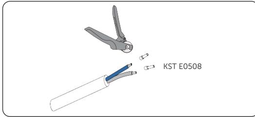
Figure 7-45 Attaching the ferrules
