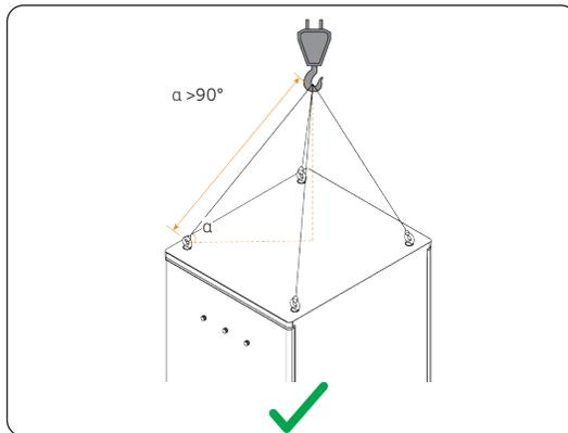
Figure 6-14 Proper way of hoisting
