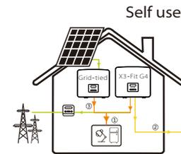
The self use mode is suitable for areas with low feed-in subsidies and high electricity prices.
