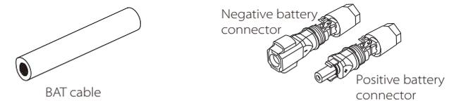
**Step 2.** Use a wire stripper to strip the 15 mm insulation layer of the wire end.
