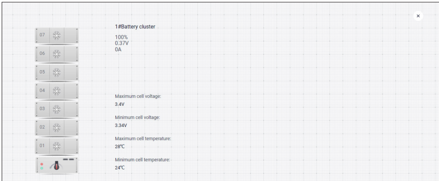
Figure 6-22 Viewing battery cluster information
